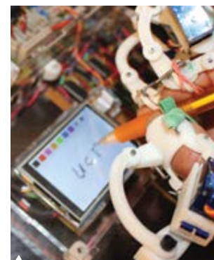
reScribe is a robotic hand exoskeleton that serves as a rehabilitation tool for stroke patients to improve their fine motor skills through task-oriented handwriting therapy.
